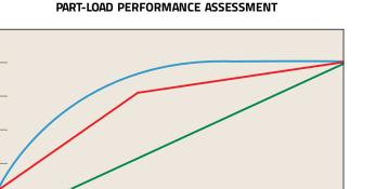
Single-Stage Lubricated Load/Unload (based on one gallon/storage per cfm)Single-Stage Lubricated Inlet Modulation with Blowdown
