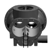
**BYPASS PORTS IN STATOR**Rotors removed to show Bypass Ports
