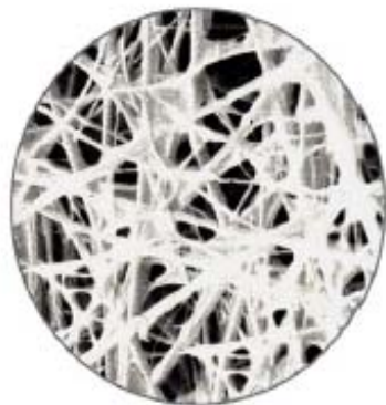
Micro-glass fiber at X500 magnification
