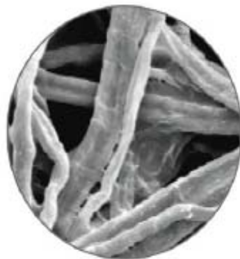
Cellulose fiber at X500 magnification
